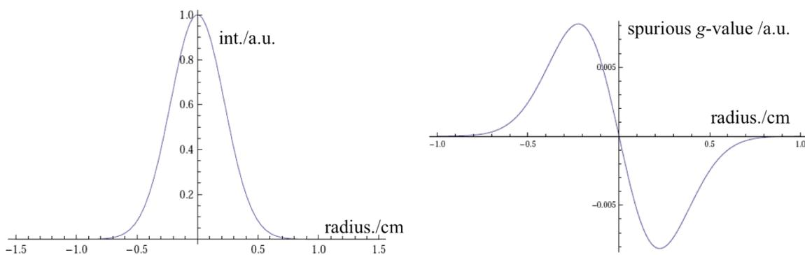
Figure 3.4 Calculated spurious  $g$ -value incurred by pointing instability. Left: distribution of laser intensity as a function of radius. We assumed a Gaussian distribution in the calculation. Right: the predicted dissymmetry factor as a function of radius, giving a pointing instability of 0.05 mrad. It is calculated by considering the lateral shift of laser spot at two extremes, and subtracting one from the other.
