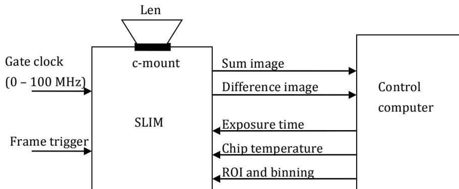
Figure 6.2 Structure of the scientific lock-in imaging module
