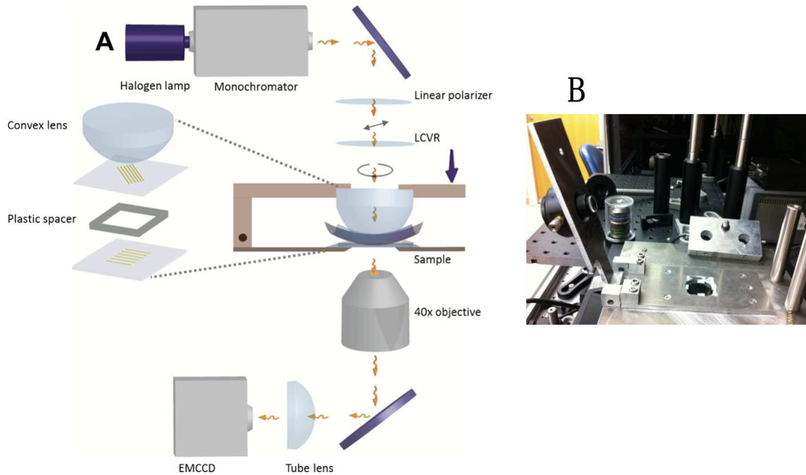
Figure 5.4 (A) Schematic of CLIC apparatus; (B) photograph of the experimental apparatus
