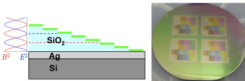
Figure 4.6 Staircase nanostructures for probing superchiral light. Left: The schematic of the structure showing transparent steps of SiO<sub>2</sub> on a reflective backing. When illuminated with monochromatic light at normal incidence, some steps will reside in a node of either the electric field or the magnetic field. Right: Photograph of a device we made with 64 steps.
