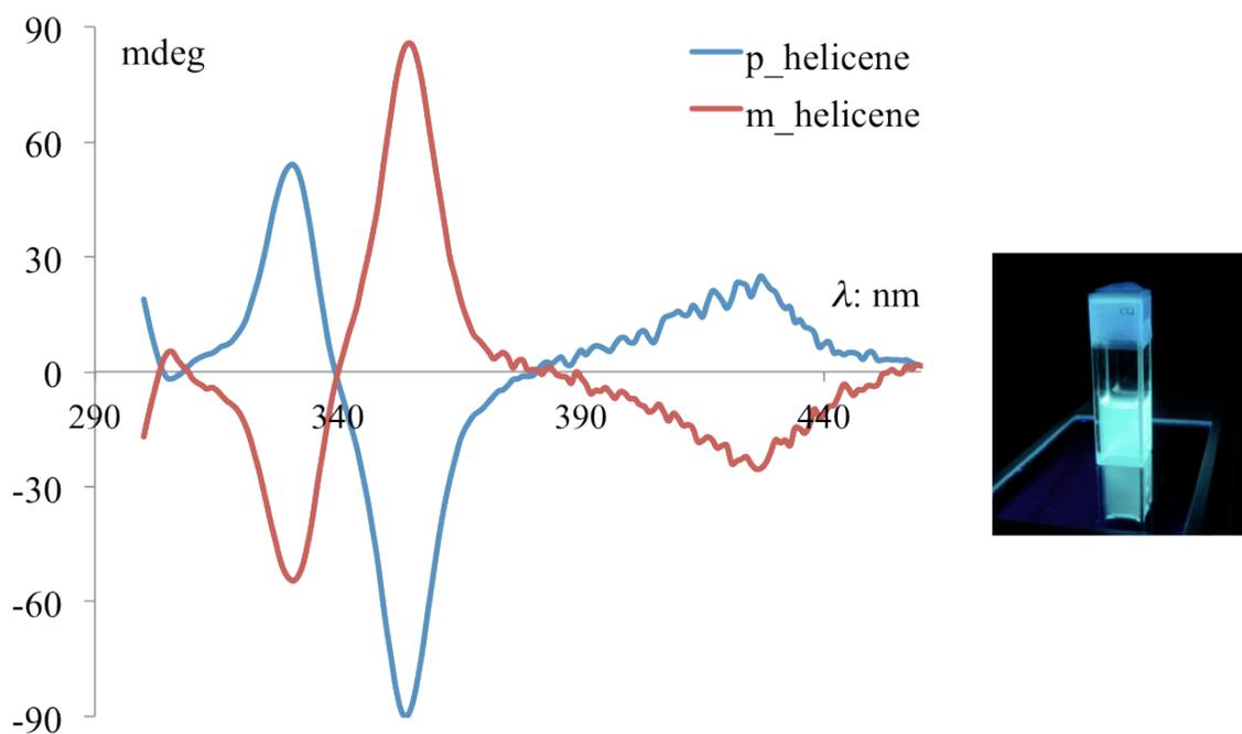
Figure 3.9 CD spectra of p- and m-triarylimine helicenes. Inset is a fluorescent image of helicene molecules under 355 nm excitation.
