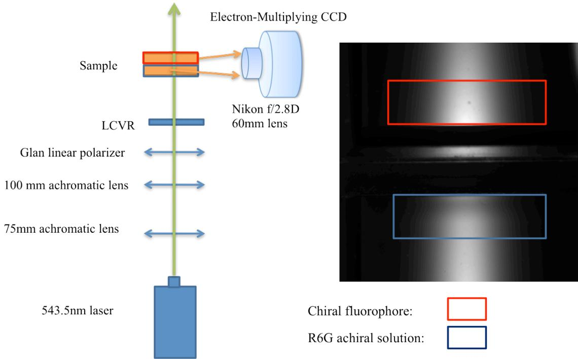
Figure 4.2 Left: the Experimental setup for sideways FDCD measurement; (B) a photo of two cuvettes, the up is filled with binaphthyl perylene dimers, and the lower is filled with achiral control molecules
