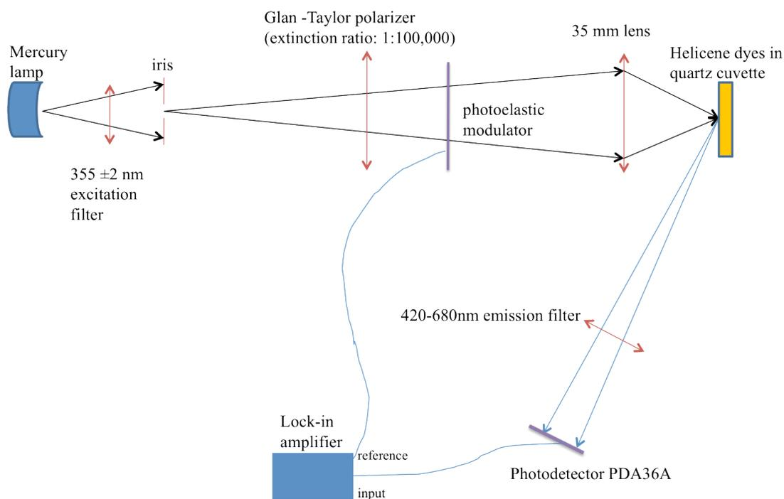
Figure 4.1 The experimental setup for PEM-based FDCD measurement
