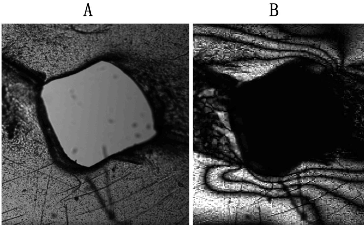
Figure 6.3 Lock-in imaging on a thin plastic sheet. (A) A sum image by SLIM after 500 frames average. The image records transmitted intensity through the sample. The square in the middle is a hole on the sample. (B) A differential image by SLIM after 500 frames average. It reports the distribution of linear birefringence within the sample.
