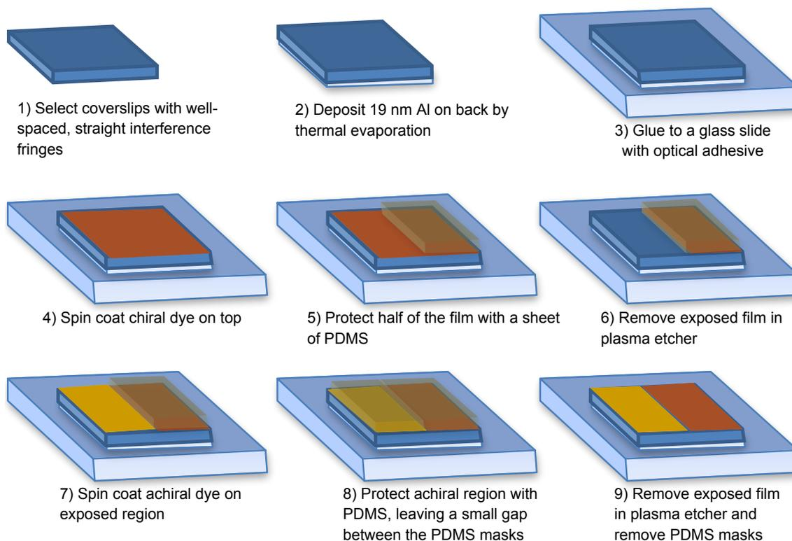
Figure 4.9 Procedure for preparing the nanometer-scale sandwich geometry
