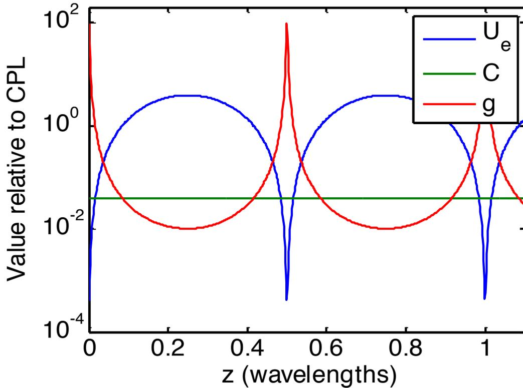
Figure 2.1 Enhanced chiral asymmetry in superchiral light. The intensity (blue) is modulated in a standing wave, while the optical chirality (green) is not. The ratio  $C = U_e$ , which determines the enantioselectivity (red), becomes large near a node in the standing wave. For this example,  $E_2 = 0.98E_1$ , and each quantity is plotted relative to its value for a single CPL plane wave.
