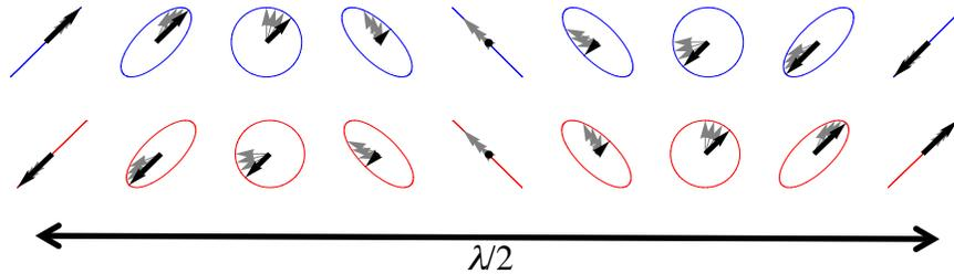
Figure 6.1 Electric and magnetic fields in the “field gradient” configuration. The fields are shown at intervals of  $\lambda/16$ . The fields lie in the plane perpendicular to the axis of propagation, but for illustration purposes each slice of the EM fields has been rotated to lie in the plane of the paper. The gray arrows represent the recent past positions of the field vectors.
